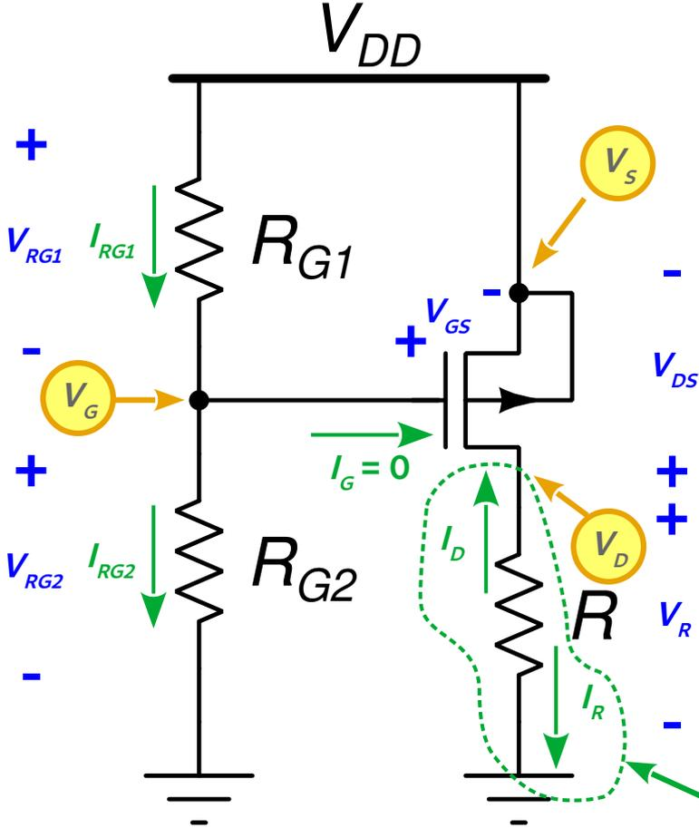
$$M1: V_{DD} - V_{RG1} - V_{RG2} = 0$$
